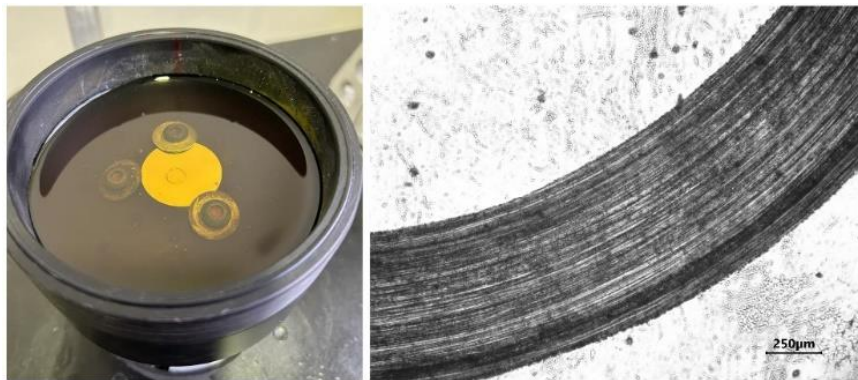
Figure. Lubricated wear of the specimen and optical micrograph
