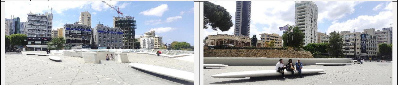
Visible are distinctive seating elements, ground lighting elements, street lighting elements, observation balconies, staircases, ramps, and tactile paving designed to accommodate disabled pedestrians.
