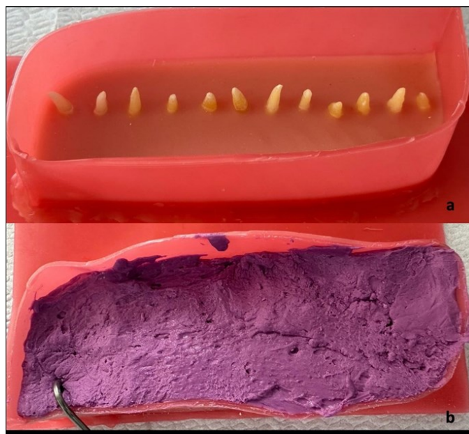
Figure 1. Stages of the setup. a: Setup of the samples before alginate placement; b: Setup of the samples after alginate placement.
