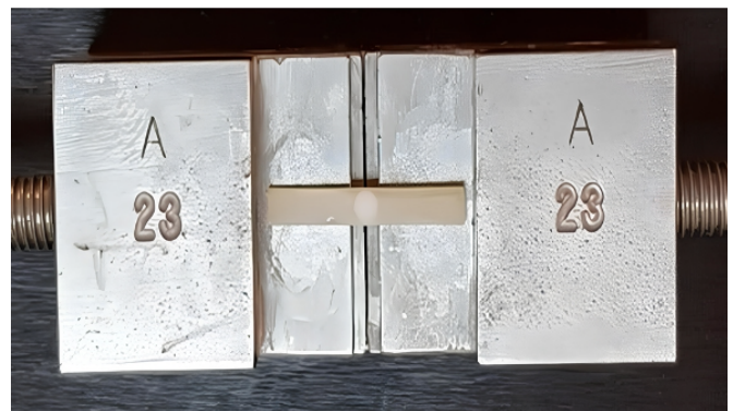
Figure 1. Applying tension to specimens in a microtension testing machine.
