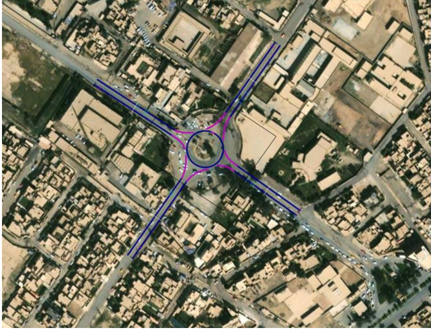
Figure 1. Illustration of the geometric layout and design features of the selected roundabout in Kirkuk, Iraq. Sources: PTV VISSIM Model.
