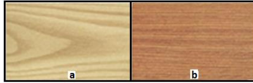
Şekil 3. Kaplama kesiş yöntemlerine göre desenli (a) ve frize (b) kaplama (Plain cut (a) and rift cut (b) veneer according to cutting methods of veneer)
