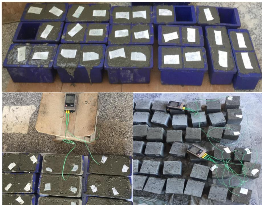
**Figure 3.** Placement of the temperature measuring device.
