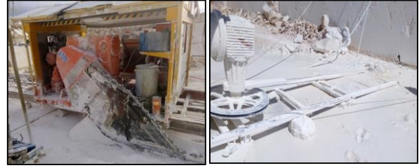
Şekil 12. Arka kesimde zincirli kollu kesici makinesinin ve alt kesimde elmas tel kesme makinesinin kullanımı (The use of chain saw machine for the back cutting and diamond wire cutting machine for the underside cuts)
