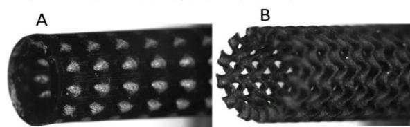
**Figure 17.** Schwarz model image (A) Gyroid model image (B)
