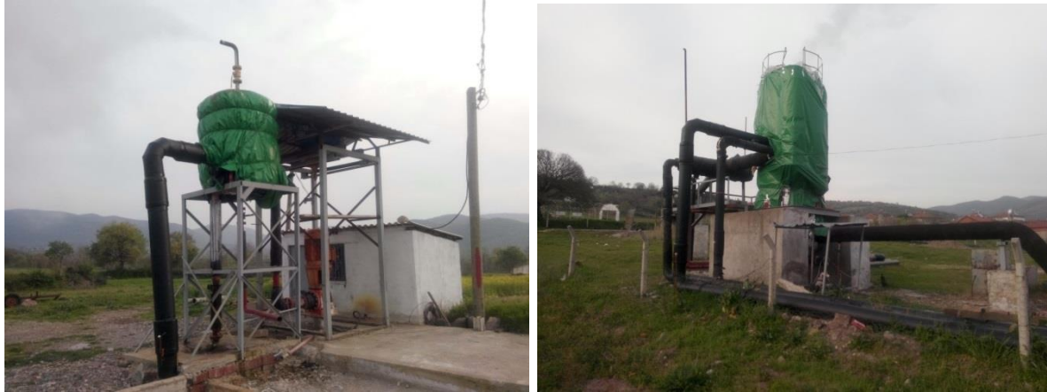
Figure 2. Views from the HK-8 well (left) and main gas separator and collection lines (right).
