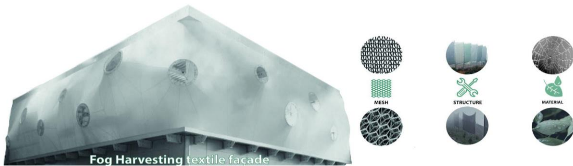
Figure 6. Web system designed as a textile product that collects water from fog [58]
