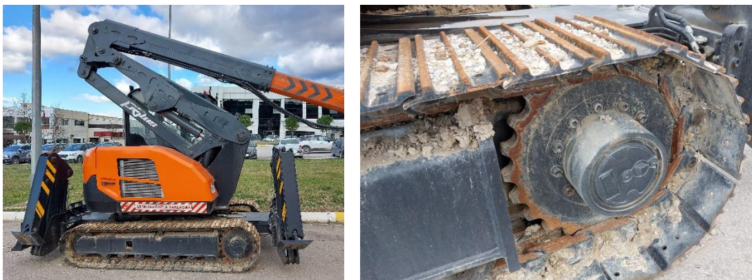
Figure 1. General view of the steel track undercarriage system (Courtesy of Smart İş Makinaları San. Tic. A.Ş.).
