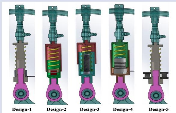
Figure 2. Transducer designs.
