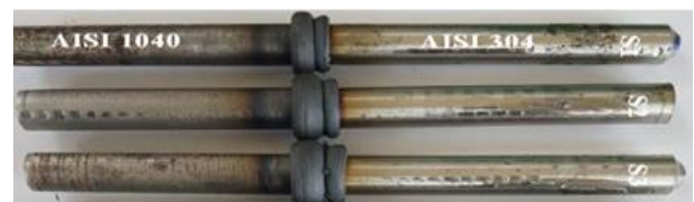
Figure 2. Macro-photograph of the friction welds
