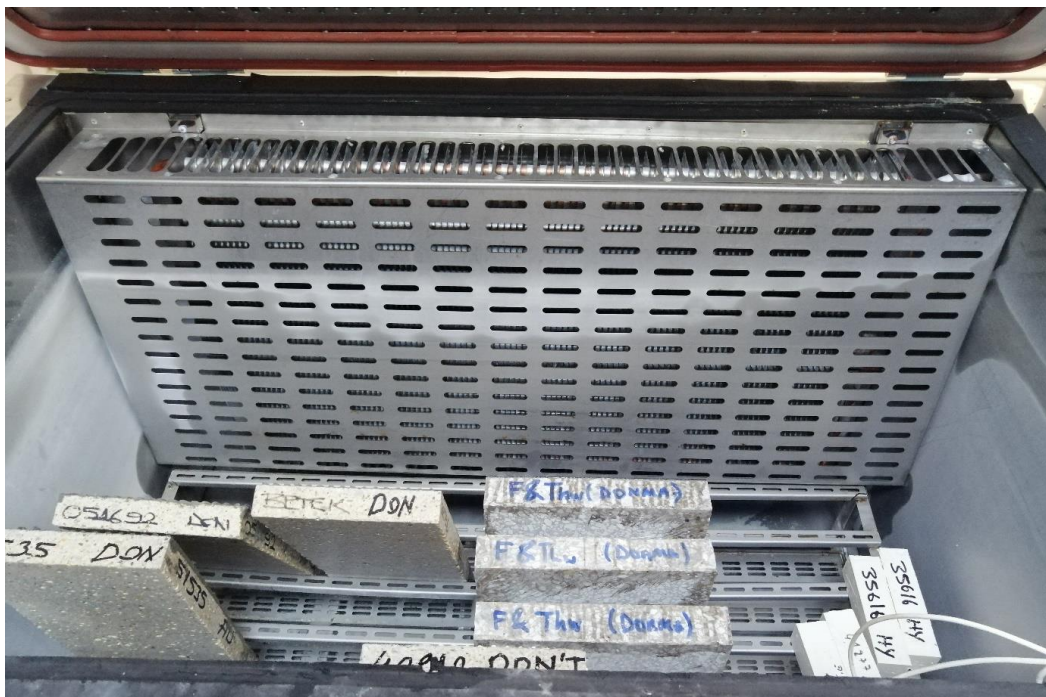
Figure 8. Test Samples placed in Freeze-Thaw Cycle Testing Machine
