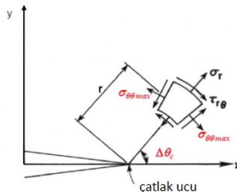
Fig.1 Stress field near the crack tip of an isotropic elastic material
