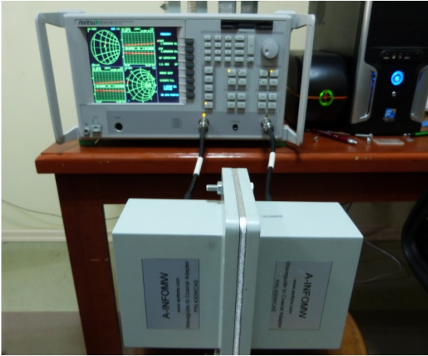
Figure 2. Photograph of the waveguide measurement system
