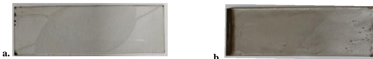
Figure 2. Images of surfaces produced on glass slide substrates by a. spin coating method and b. dip coating method.
