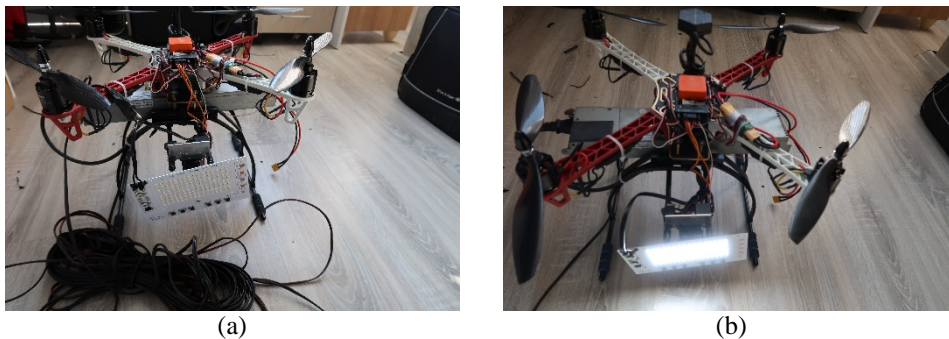
Figure 6. (a) System configuration with mounted AC cables (b) Operational system with active projector
