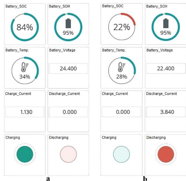
Figure 10. Arduino IoT Cloud mobile interface; a) Charging time, b) Discharging time.
