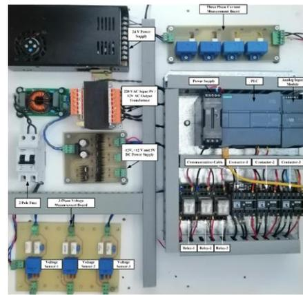
Figure 6. Experimental setup (Denedy dzeneyi)
