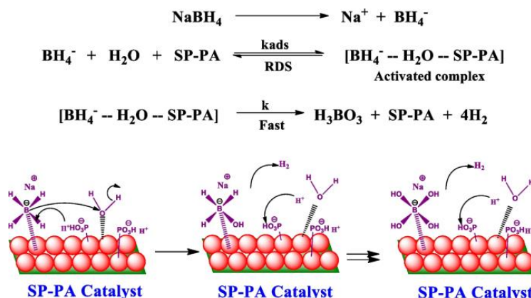
Figure 9. Catalytic hydrolysis of NaBH 4 for H 2 production catalyzed by phosphorylated silica particles (SP-PA) (Ganesan et al., 2022[37]).
