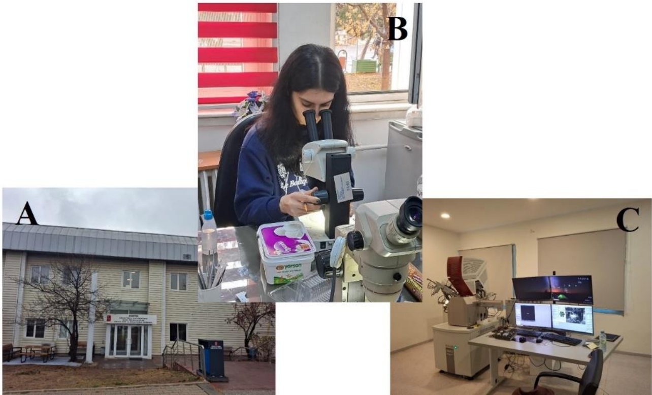
Figure 2. A. Hacettepe University Advanced Technologies Application and Research Center, from which we provided the SEM images; B. SZX7 Stereo Microscope, from which we removed the sample genitals; C. Tescan Brand GAIA3+Oxford XMax 150 EDS model Electron Microscope, from which we obtained the SEM images.
