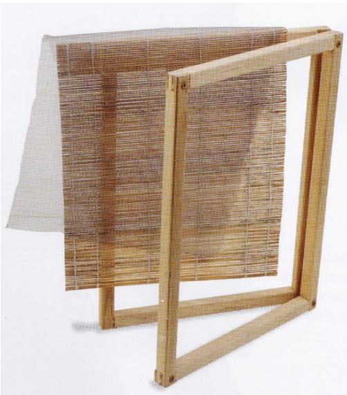
Figure 1. Mould for the manufacture of Japanese paper. The mesh is always glazed and goes independent of the frame. Image obtained from: Asunción, Josep. The Paper. Techniques and traditional methods of production . Editions Parramón. Barcelona, 2009:63
