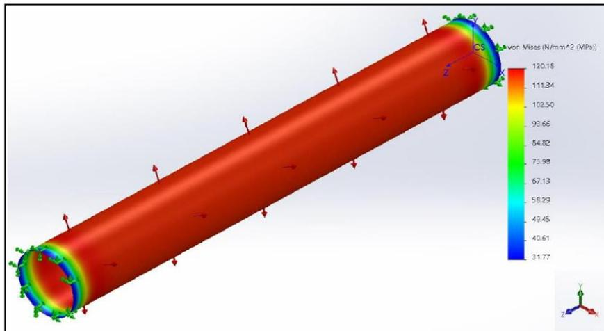
**Figure 3.** Strength value of +75°, 90°, -75°, 90° CFRP wound cylinder.
