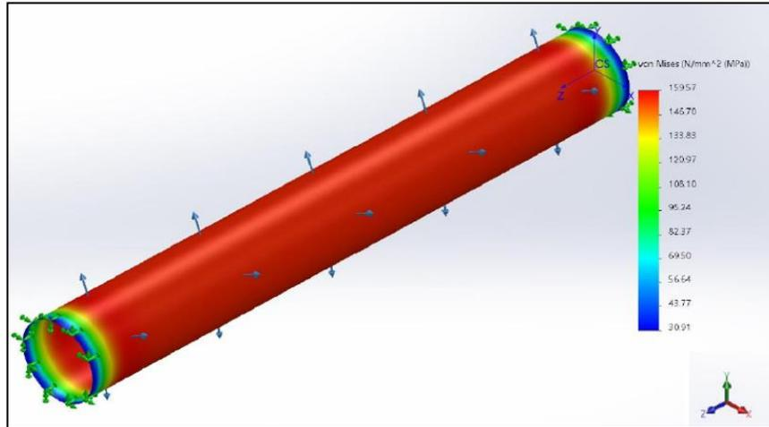
**Figure 2.** Strength value of +45°, 90°, -45°, 90° CFRP wound cylinder.
