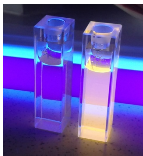
Figure 1. Fluorescence photograph of Tr1 in pure DMSO (cell on the left) and in DMSO/ \text{H}_2\text{O} mixture (cell on the right).
