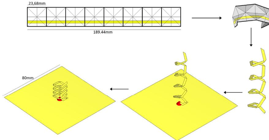
**Figure 2.** Origami folding based helix antenna design
