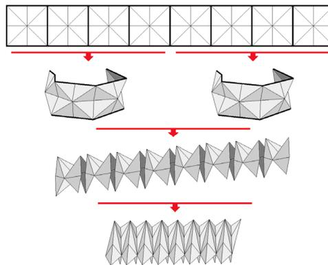
Figure 1. Origami folding technique to design helical accordion
