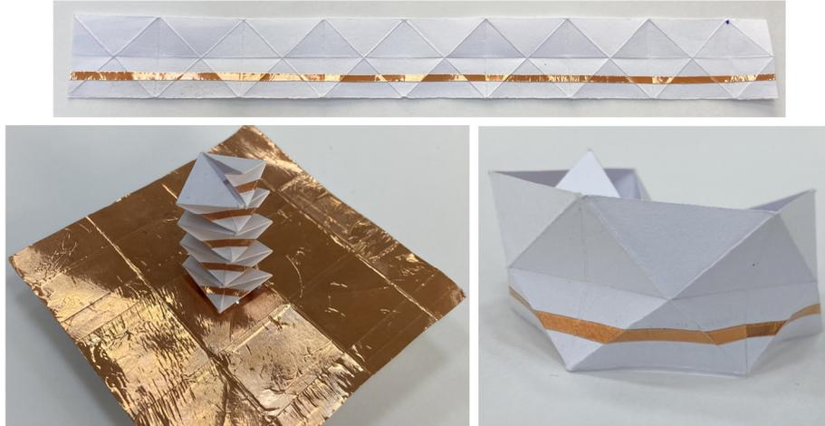
**Figure 6.** Fabricated accordion-like origami helix antenna
