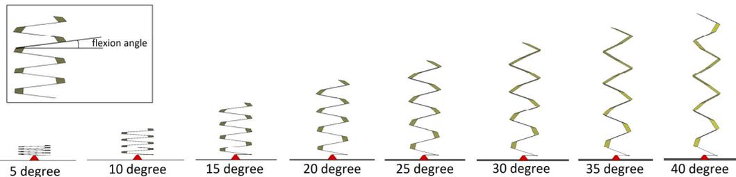
**Figure 3.** Helix antenna variations versus various flexion angle
