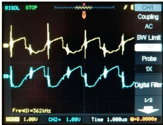
Figure 13.a Gate signals of MOSFETs under energized
