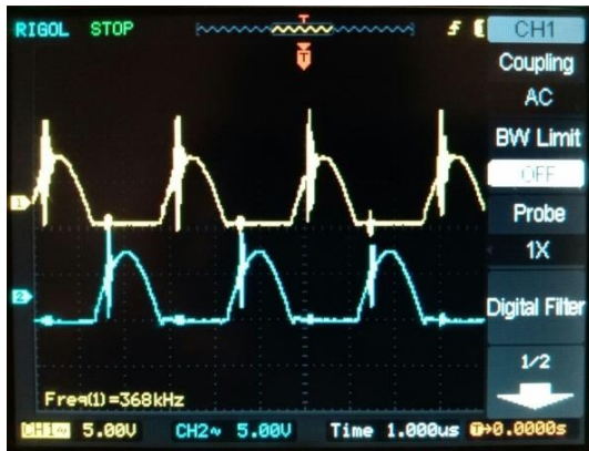
Figure 13.b Drain voltages on MOSFETs during the running
