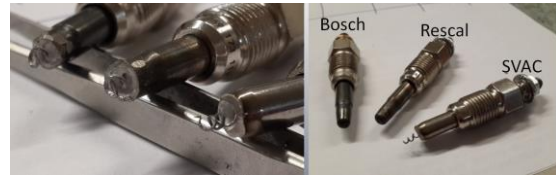
Figure 5. Three kinds of glow plugs after cut the ends of the heating area
