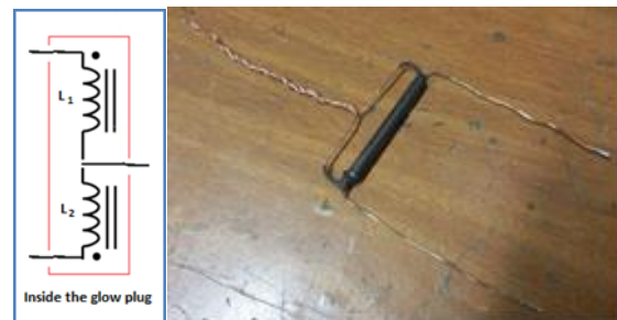
Figure 9. The center tapped coil to simulate glow plug
