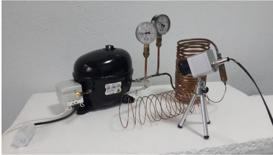
Figure 2. Prototype snow accumulation device and test setup
