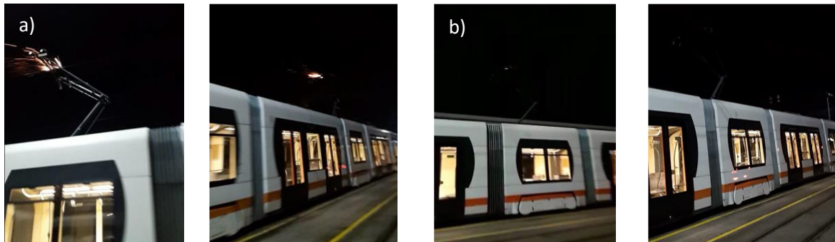
Figure 7. Observed arc formation in field tests a) Reference b) % 100 Mono-ethylene Glycol
