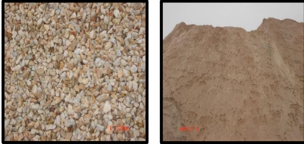
Fig. 2. Elazığ province calcareous aggregates in the quarry; (a) coarse aggregate, (b) fine aggregate (Tuğrul, 2015)
