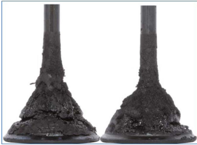
Figure 3. A ford intake valves after 190 km way spent [15].
