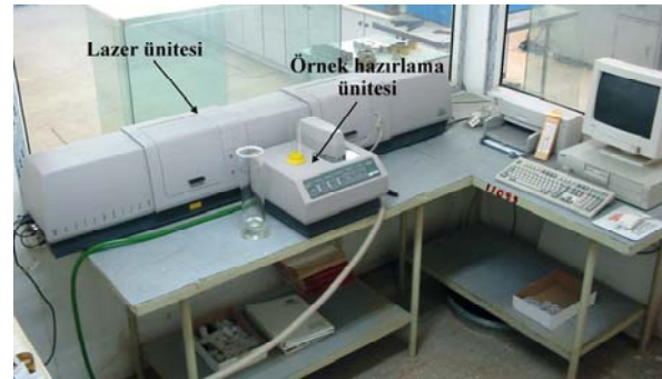
Şekil 3. Malvern Master SizerX-Long Bed Lazer kırınım cihazı.(Malvern Master Sizer X-Long Bed laser diffraction instrument)
