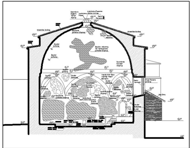
Fig. 4 Ceiling surveying drawings and A-A cross section
