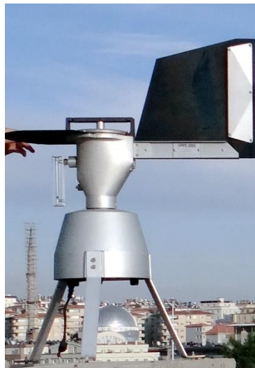
Figure 1. Hirst-type pollen and spore trap (Lanzoni VPSS 2000)
