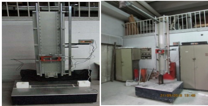
Figure 2. (a) Weight Drop Test Setup and Settlement of Sample to the Fixture
