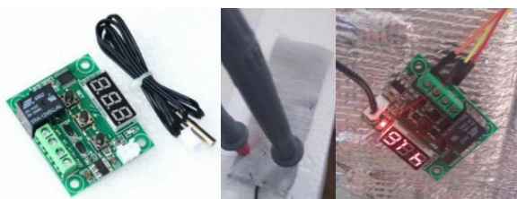
Figure 2. Temperature meter, sensor and measuring device
