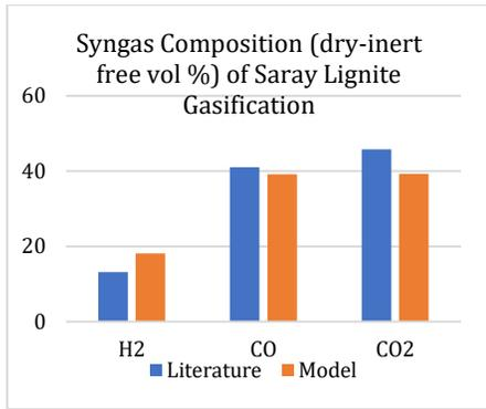
**Figure 3.** Comparison of syngas composition between literature and model
